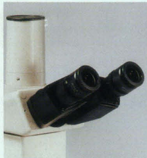
Multiple image ports include side, front, and optional trinocular eyepiece tube.
