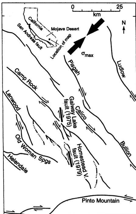
**Fig. 3.** The nearly fault-normal orientation of the Mojave compression to the older faults and its optimal orientation to the Homestead Valley and Galway Lake ruptures, which suggests the emergence of a new fault line caused by the gradual locking of the older faults. [Reprinted from (7)]
