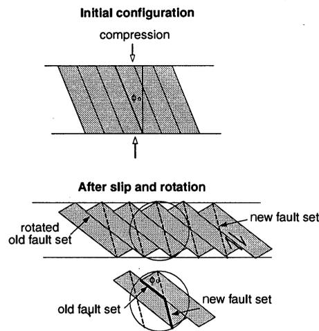
**Fig. 4.** The origin of kinks. When blocks and their bounding faults rotate away from the direction of compression or shortening, they eventually lock up. Further deformation requires that a new set of faults develop. When the new faults begin to develop and the old ones begin to lock, slip can occur simultaneously on both, leading to kinked slip, as illustrated by the heavy line.
