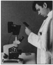
posure and filtration control system to produce high-quality instant color and black-and-white prints with push-button ease. The camera attaches to a microscope by sliding its built-in ×10 magnification lens directly into the microscope's eyepiece tube or phototube. Weighing only 2.2 pounds with dimensions 8 by 7 by 7 inches, it can be moved from microscope to microscope to serve as the imaging system for an entire laboratory. Polaroid. Circle 140.
