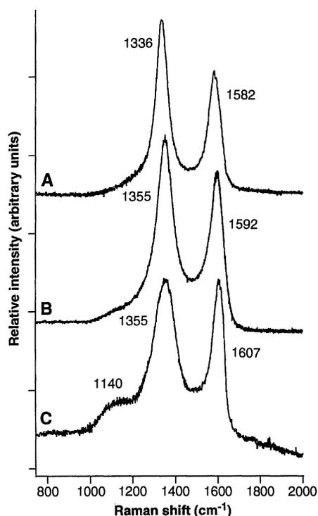
**Fig. 3.** Raman spectra of (A) the transparent carbon produced by pyrolysis of **1**, (B) the carbon produced by pyrolysis of **2**, and (C) the black, reflective carbon produced by the pyrolysis of **1**.
