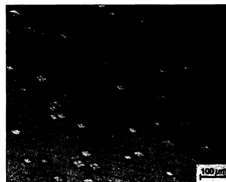
"Spontaneous fission tracks in muscovite after etching in 40% [hydrofluoric acid] for 15 h at 25°C." [From Fission-Track Dating ]
