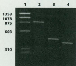
PCR amplification of the 5' ends of the human transferrin receptor (Lane 2: 0.87 kb. Lane 3: 0.45 kb) and tissue-type plasminogen activator genes (Lane 4: 0.40 kb).
