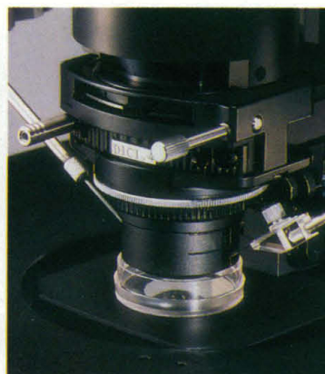
0.85 and 1.4 N.A. DIC condensers for high resolution, high magnification microscopy.
