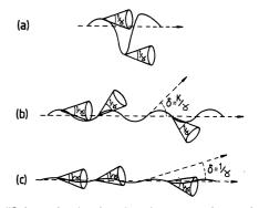
"Schematic showing the electron motion and synchrotron cone emission for the three insertion devices: (a) wavelength shifter; (b) multipole wiggler; and (c) undulator." [From Macromolecular Crystallography with Synchrotron Radiation]
