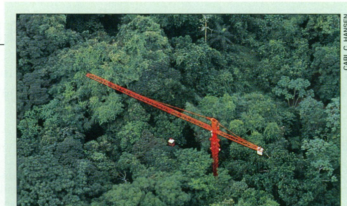
In the treetops. Crane with gondola yields unimpeded, repeatable access to area 110 meters in diameter.
