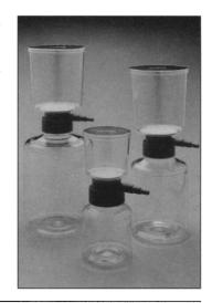
units are available with 200-, 500-, or 1000-ml receiver bottles. The filtrate can be stored in the receiver bottles so there is no need to transfer and risk recontamination of sterile solutions. Millipore. Circle 96.
