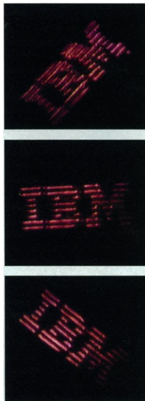
Three in one. Lighted from different angles, a single piece of "photo-refractive" plastic reveals three different images.
