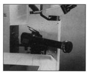
or too thick to fit onto the microscope stage. The SPRA allows the user to perform nondestructive analyses of small portions of large samples in the reflectance mode. The SPRA attaches to the nosepiece of the IR-Plan family of microscopes and can be positioned at different angles to accommodate the sample. Spectra-Tech. Circle 91.
