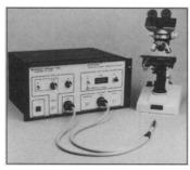
in approximately 8 s. Oxygen levels can be measured from saturation levels to less than 0.01 torr. The process can produce quantitative images of vascular oxygen concentrations as well as high-contrast qualitative images of the microvasculature. Applications include studies of oxygen delivery to tissue, metabolism of tissue, animal models of stroke and cardiovascular traumas, wound healing, and hypoxic traumas. Medical Systems Corp. Circle 93.
