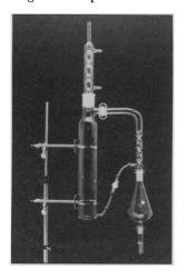
al ball and socket joints while allowing easy assembly and reducing the possibility of leakage with a vacuum-tight seal. A built-in Slow-Dry concentrator permits extraction and concentration with the same apparatus. The concentrator tube incorporates a glass jacket around the constricted bottom portion, creating an insulating air space that shields the sample within the tube and provides a temperature buffer to reduce the risk of overdrying the sample. Kontes Glass. Circle 91.
