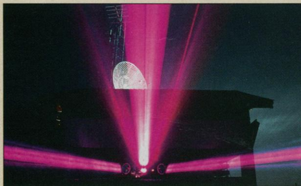
Taking the measure of Parkfield. A laser distance-measuring device watches for precursory crustal motion.
