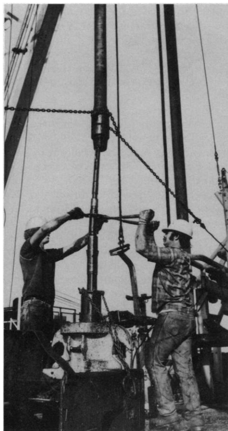
"Taking a wire-line core on Glomar Challenger . The roughnecks have already unscrewed the drill string near its upper end, and secured the core barrel to a clamp on the rig floor. Then they had to unscrew the "overshot" (a hook-like device) at the end of the sandline, which had been sent down to fish out the core barrel from the bottom of the hole. After this was done, the core barrel could be taken out of the drill string, as shown here." [From Challenger at Sea ]
