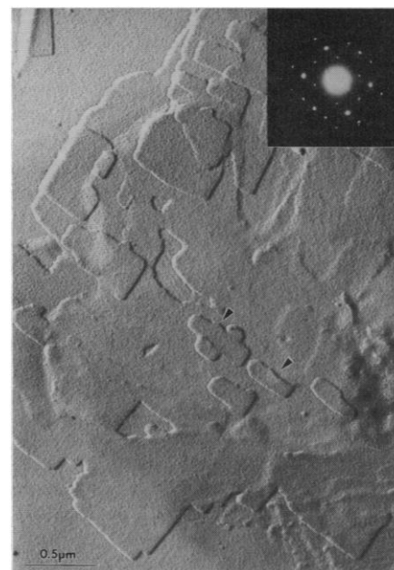
Fig. 9. Transmission electron micrograph showing stacked 2D polymers. The flat objects are less than 100 Å thick and can self-assemble into single crystals as revealed by the electron diffraction pattern in the upper right-hand corner. The arrows point to supramolecules that are fractions of a micrometer in planar dimension and nanometers in thickness.
