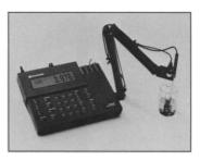
but also conductivity readings. It automatically selects the correct range of conductivity, salinity, and resistivity for the sample. The instrument tests in any two modes at once and displays the results from both electrodes simultaneously on a large liquid crystal display screen. Fisher Scientific. Circle 93.
