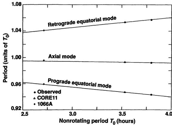
**Fig. 3.** Rotational splitting of translational triplet periods as a function of the period in the absence of rotation. The curves are branches of hyperbolas and are generated with the parameters of Earth model CORE11. Computed periods for Earth model 1066A and the observed periods are both accurately forecast. Relative errors in predicting locations of the observed resonances are 0.040, 0.027, and 0.020 percent.
