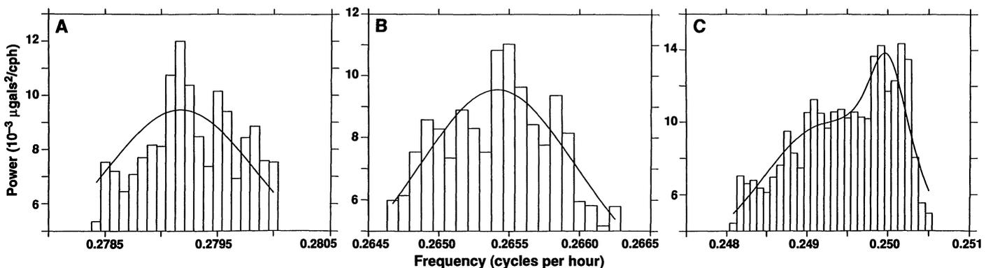
**Fig. 4.** Fitted resonance (A) for the prograde equatorial inner core translational oscillation ( $T_P$ ), (B) the axial translational oscillation of the inner core ( $T_C$ ), and (C) the retrograde equatorial translational oscillation
