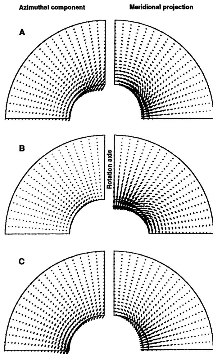
**Fig. 2.** Displacement vector fields in the fluid outer core of the three translational modes of the solid inner core. The azimuthal components are shown in perspective. (A) Retrograde equatorial mode. (B) Axial mode. (C) Prograde equatorial mode. In each case the azimuthal component leads the meridional component by  $90^\circ$ .
