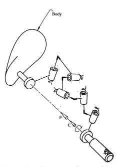
"A wrench applicator across five screw joints which is almost certainly unstable. The joints are merely arranged as members of a 5-system of motion screws whose reciprocal 1-system is the required wrench. If the screw joints were all simply hinges, namely screw joints of zero pitch, the hinge axes would belong to the same linear complex whose pitch would be the pitch of the wrench." [From Freedom in Machinery, vol. 2]
