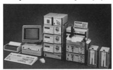
up biological or food samples, and immediately injects each sample into a reversed-phase high-performance liquid chromatography column coupled with fluorometric detection. After derivitization, the system removes all interfering macromolecules and undissolved substances that can adversely affect column performance. Because the fluorophores are prepared just before injection, results are not affected by the rapid fluorescence decay of certain derivatives. Gilson Medical Electronics. Circle 441.
