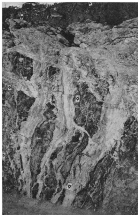
Fig. 1. The fracture system filled with layered calcite and silica, exposed on the south wall, east end of Trench 14. The trench wall is about 3.5 m high.
