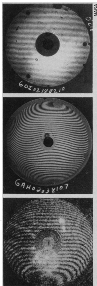
Ignored. The mirror looked great to the reflective null (top)—but not to the inverse and refractive nulls (middle and bottom.)
