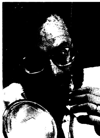
No sweat. A GE engineer examines the heat-reflective inner bulb of a halogen lamp.
