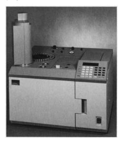
injector ports, which allows unobstructed access to the ports without removal of the autosampler. The system's three speeds of injection and five GC methods can be programmed through the keyboard. Two separate automation modes can also be programmed, so that individual runs can be performed with different columns and under various conditions. Perkin-Elmer. Circle 505.
