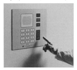
free of crevices that can trap particulate matter. An integral speaker-microphone replaces the telephone handset. The phone also features an "auto answer" capability, allowing users to remain at their stations while answering calls. GAI-Tronics Corp. Circle 468.
