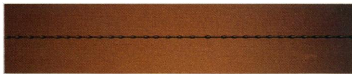
Fig. 2. Drops resulting from a thin film of silicone oil coating a nylon fiber (radius b = 80 \mu\text{m} ). The spacing between the droplets is regular and is about 10b (as shown by Rayleigh) for thin films on fibers.
