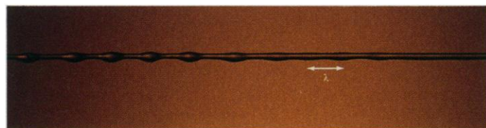
Fig. 1. Film of honey on a fishing line of radius b = 140 \mu\text{m} . The film is made by drawing the thread horizontally out of a large drop of honey. The instability is fully developed on the left, but still not on the right where the optimal wavelength \lambda has not yet been selected.
