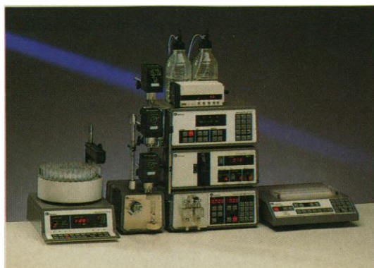
HPLC DfB System Prep 10 dedicated for optimal peptide purification and analysis
