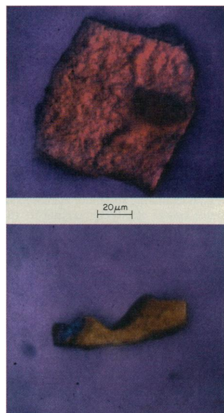
Fig. 2. Photographs of an \text{AlPO}_4 berlinite sample taken between crossed polarizers (white transmitted light with gypsum plate) before compression (top) and after decompression from 28 GPa (bottom). After quenching, except for the left end where part of the sample flaked off (hence is thinner), the interference color is uniform, implying that the sample is a single crystal with uniform orientation across its entire width. The apparent difference in the color of the crystal before compression and after decompression is an artifact of the photography. The scale bar is 20 \mu\text{m} long.
