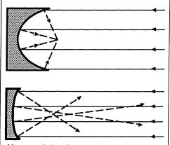
**Aberrant behavior.** A perfect parabolic mirror will reflect every ray of starlight to a single focal point (top). But Hubble's mirror isn't perfect, the rays do not cross at a single point, and so there is no perfect focus (bottom).
