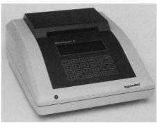
and customization of protocols. A sample temperature sensor monitors conditions and provides real-time feedback to control the system. The Microcycler E is available in two models, one for 0.5-ml and one for 1.5-ml microcentrifuge tubes. Eppendorf. Circle 507.
