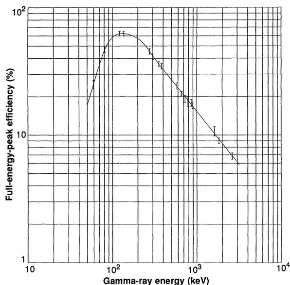
**Fig. 4.** Full energy peak efficiency of the detector as a function of gamma-ray energy. The error in the efficiency is the combined errors of the count rate, the background rate, the activity of the source, and the branching ratio to 1 SD.
