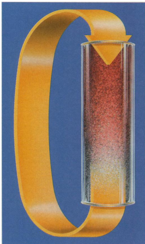
With continuous flow, activated amino acids are introduced into the system and recirculated through a packed bed reactor. The bed's inherent low volume maintains high amino acid concentration during coupling.
