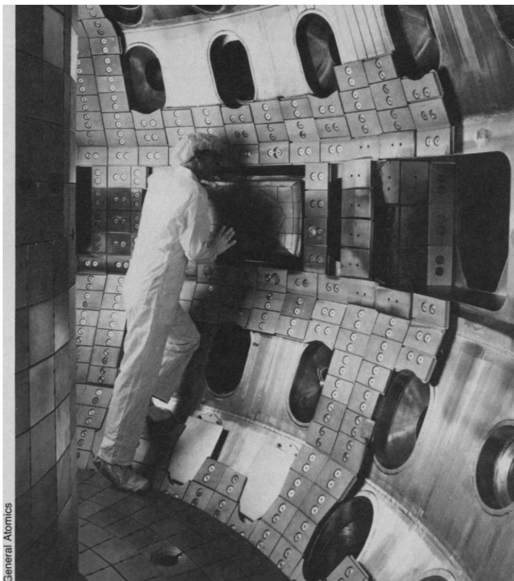
Idle fusion reactor. A technician inspects heat shielding tiles on the outside wall of the Doublet III-D tokamak at General Atomics in San Diego, California.
