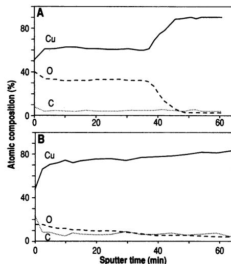
**Fig. 6.** Surface composition depth profiles of Cu powder (75- $\mu$ m mean diameter) before and after ultrasonic irradiation. Depth profiles were derived from Auger electron spectra; sputtering times correspond to an erosion rate of  $\sim 270$  Å/min. The upper depth profile is before ultrasonic irradiation; the lower after 4 hours of irradiation in dimethylformamide at 15°C. [Reprinted from (43) with permission © American Chemical Society]
