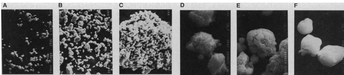
**Fig. 5.** The effect of ultrasonic irradiation on the particle agglomeration and surface morphology of Ni powder. High-velocity interparticle collisions caused by ultrasonic irradiation of slurries responsible for these effects. Note the magnification of the upper scanning electron micrographs is tenfold less
