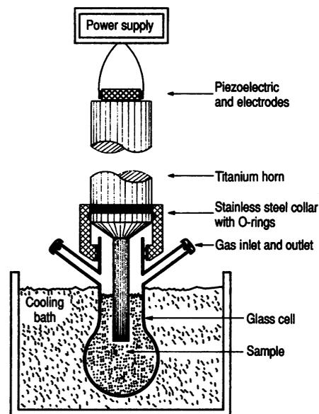
**Fig. 2.** A typical sonochemical apparatus. Ultrasound can be easily introduced into a chemical reaction with good control of temperature and ambient atmosphere. The usual piezoelectric ceramic is PZT, a lead zirconate titanate ceramic.
