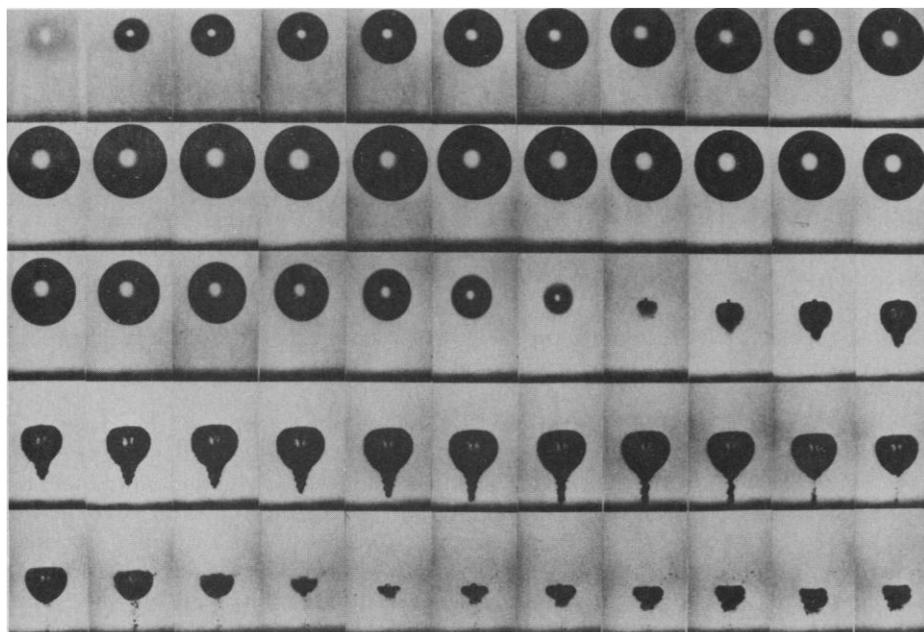
**Fig. 4.** Cavitation near a liquid-solid interface. High-speed microcinemagraphic sequence of laser-induced cavitation near a solid surface, showing the formation of a microjet impact; 75,000 frames per second. [Photograph courtesy of W. Lauterborn; reprinted from (29) with permission © Annual Reviews]
