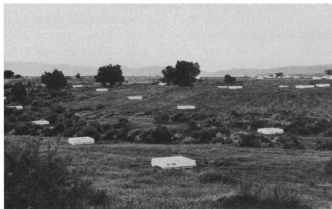
Fig. 3. Photograph of a portion of the Chicago air shower array at Dugway, Utah (courtesy of J. Cronin).
