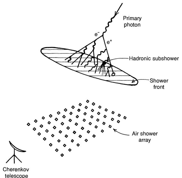
**Fig. 2.** This sketch shows an air shower generated by a primary photon of energy  $\sim 50$  TeV or higher as it approaches an air shower array. This example includes a single hadronic subshower in which a photon produces pions, some of which decay to muons. The muons can penetrate to trigger shielded detectors. A Cherenkov telescope can detect signals from showers of lower energy ( $\sim 1$  TeV) in which the particles are absorbed before they reach the level of the detector.
