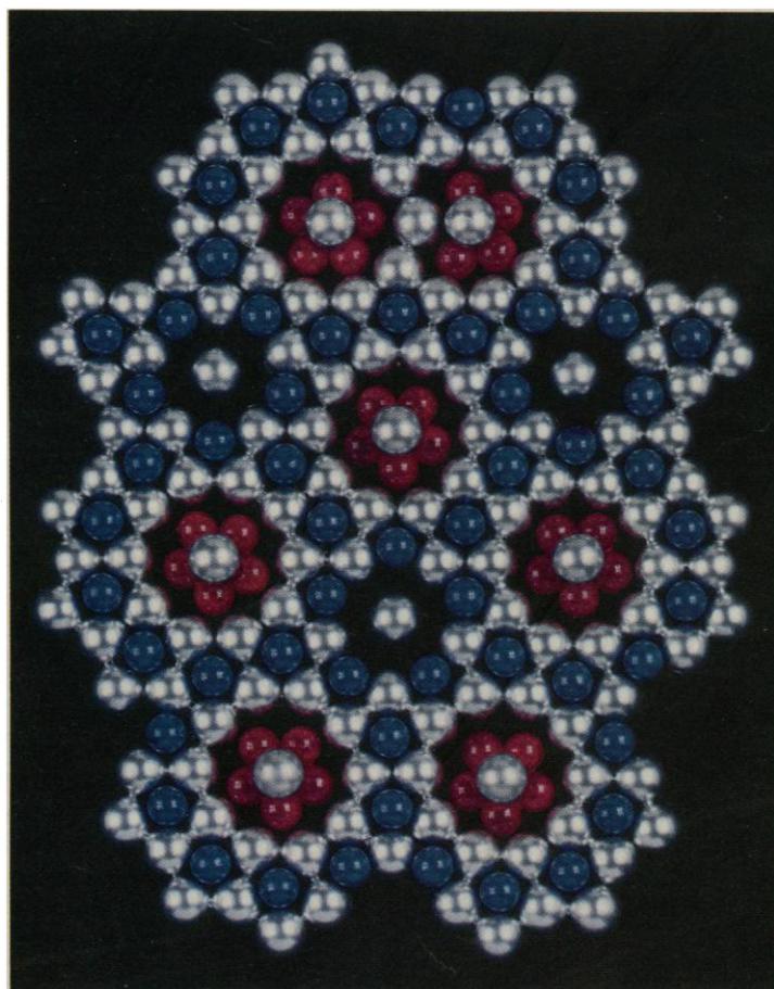
Fearful symmetry. Model of a quasicrystalline material in which the silver balls represent aluminum atoms, the blue cobalt atoms, and the red copper atoms.
