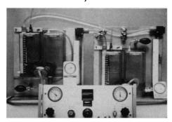
variety of in vivo conditions. All stock models come with integrated flow meters and arterial pressure gauges. The systems are appropriate for cardiac assist research, prosthetic valve evaluation, studies of circulatory system interrelationships, and the calibration of standard flow transducers. The manufacturer also produces a variety of blood pumps for in vivo and in vitro use. Cardiac Systems. Circle 449.
