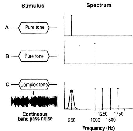
**Fig. 1.** Scheme of the stimulus conditions in (left) time- and (right) frequency-domain representation. (A) Pure-tone burst of 250 Hz (spectral pitch stimulus); (B) pure-tone burst of 1000 Hz (spectral pitch stimulus); (C) complex-tone burst (virtual pitch stimulus) consisting of the fourth through the seventh harmonic of 250 Hz, presented simultaneously with narrow-band noise centered at 250 Hz.
