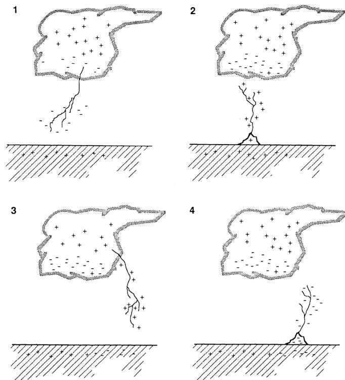
**Fig. 3.** Categorization of the four types of lightning between cloud and ground. Category 1 lightning begins with a negatively charged leader moving downward; category 3 discharges are initiated by a downward moving positive leader. Category 2 lightning has a positively charged leader, and hence this type effectively lowers negative charge to earth; category 4 has a negatively charged leader and effectively lowers positive charge. [Reprinted from (21) with permission, © 1987 Academic Press]
