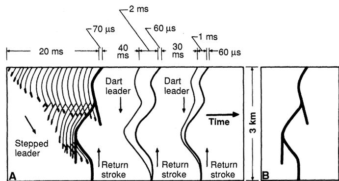
**Fig. 6.** (A) Luminous features of a lightning flash below cloud base as would be recorded by a streak camera. Increasing time is to the right. For clarity the time scale has been distorted. (B) The same lightning flash as would be recorded by a camera with stationary film. [Adapted from (21) with permission, © 1987 Academic Press]
