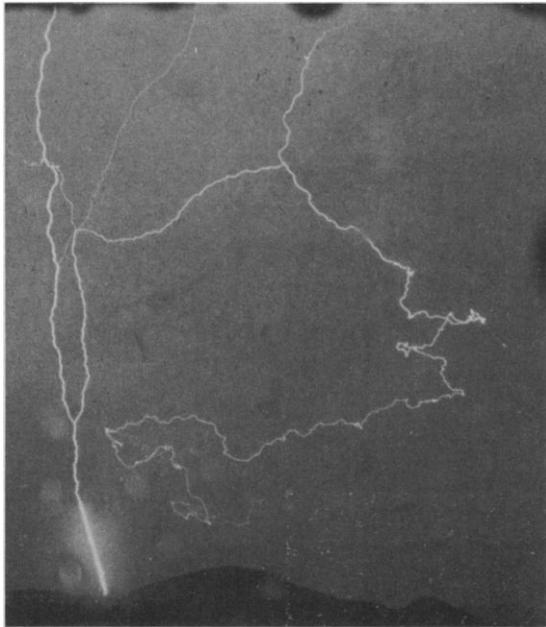
**Fig. 8.** Rocket initiated lightning. The straight part of the channel at the bottom is caused by the wire between the rocket and ground. Courtesy of P. Hubert. [Reprinted from (21) with permission, © 1987 Academic Press]
