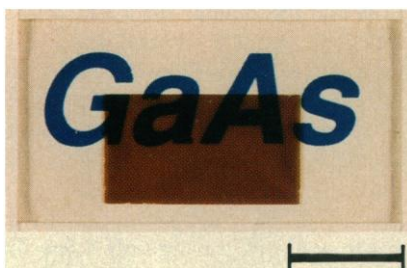
Fig. 5. The epitaxial liftoff films can be bonded directly to glass by natural intermolecular forces. A 1500 Å thick \text{Al}_{0.3}\text{Ga}_{0.7}\text{As}/\text{GaAs}/\text{Al}_{0.3}\text{Ga}_{0.7}\text{As} double heterostructure on a glass slide appears transparent with a brownish tint. The length marker is 1 cm.
