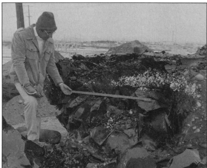
Contaminated soil that has been melted on location and converted into a stable, glass-like substance in a test at Pacific Northwest Laboratory.
