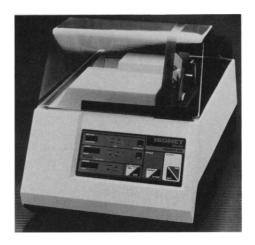
hard materials. The unit features a corrosion- and impact-resistant molded cabinet with see-through hood, electronic touch-pad controls with light-emitting—diode readouts, fully electronic automatic operations, variable load application, a sensing circuit that returns the sample arm to a raised position upon completion of a cut, a precision micrometer with a digital readout for positioning parts to be sectioned, and a built-in coolant-lubricant recirculating system. Buehler Ltd. Circle 467.
