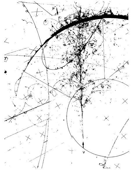
Fig. 2. A typical neutrino event as observed at the Big European Bubble Chamber filled with neon at the CERN 450-GeV super proton synchrotron accelerator. The muon may be seen at the left; it has been tagged by an external muon identifier. The many-particle hadron shower is to the right.
