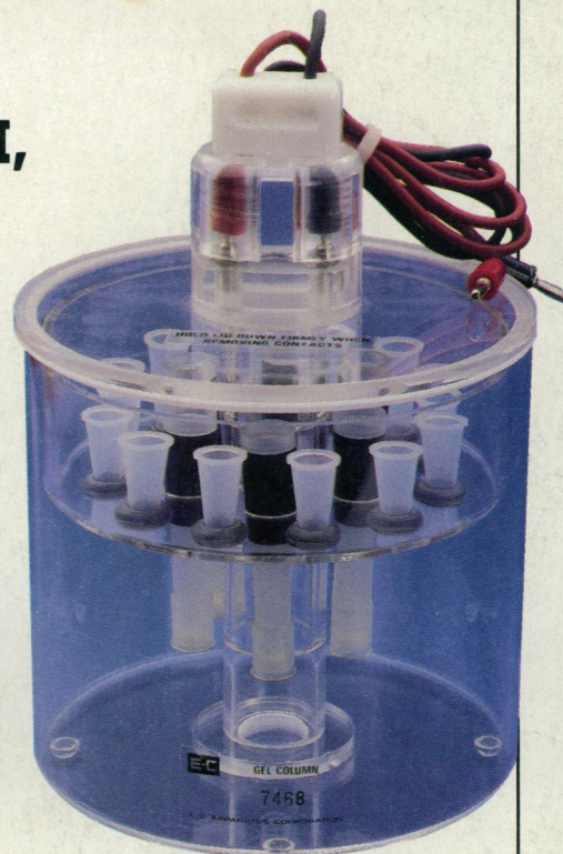
EC341 Geluter® II with fixed disposable columns in place; connects to any power supply.
