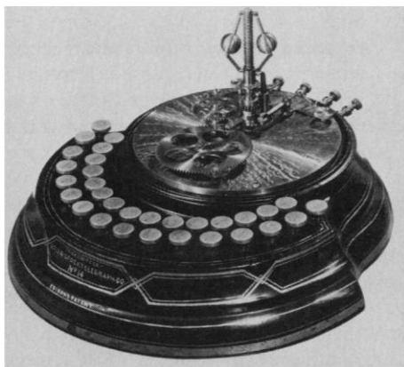
Transmitter for printing telegraphs constructed at Edison's shop in New York (around 1871), embodying Edison's U.S. Patent 131,343. [From The Papers of Thomas A. Edison , vol. 1]
