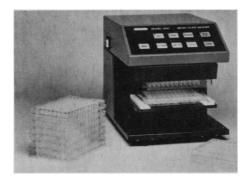
each plate is raised to the same position. In the automatic mode, the 1550 can dispense 100 to 300  $\mu$ l of wash fluid to each well, can allow soaking from 2 to 128 s, and aspirates the contents of the plate; the cycle can be repeated three to five times. An overflow tube at the rim of each well prevents cross contamination. Wash solution is pumped into the washer, not fed by gravity. Bio-Rad Laboratories, Chemical Division. Circle 446.
