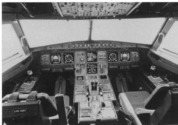
A320: The pilot's view. Mechanical dials and gauges have given way to color CRTs; "steering wheels" have given way to sidestick controllers.
