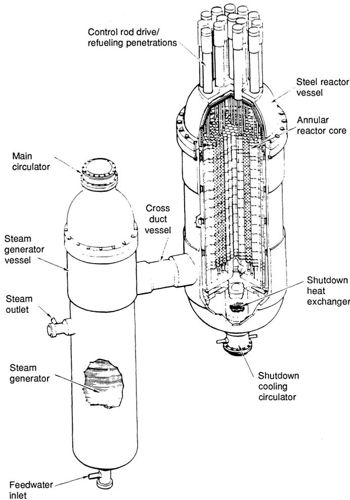
Fig. 6. MHTGR side-by-side arrangement with prismatic fuel.
