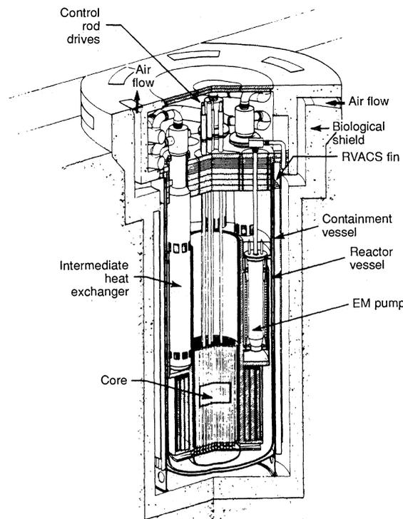
Fig. 5. PRISM reactor module. EM, electromagnetic.
