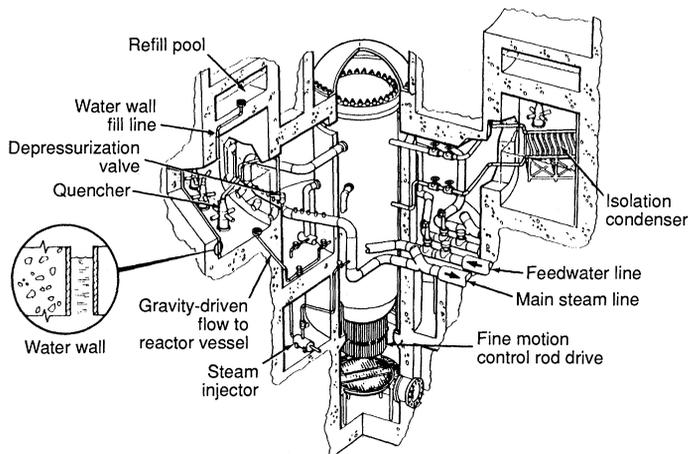
**Fig. 3.** Features of the passively stable PWR.
