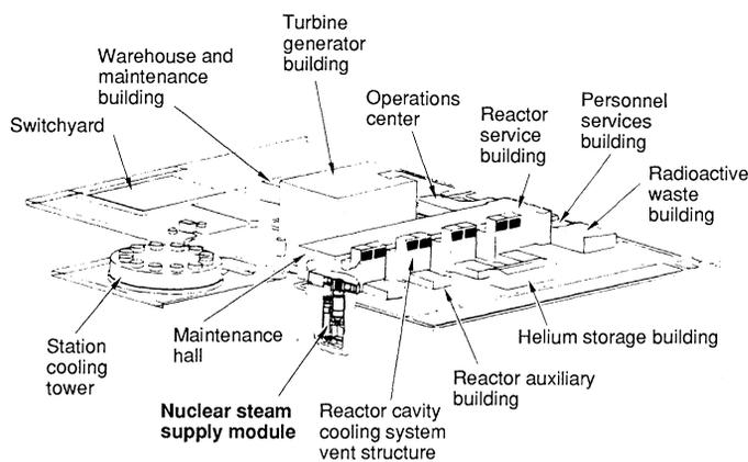
Fig. 7. Reference four-module MHTGR plant.
