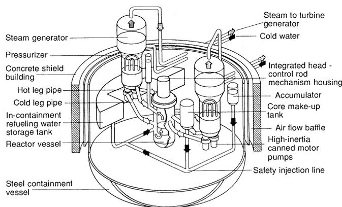
Fig. 1. Advanced passively stable PWR.
