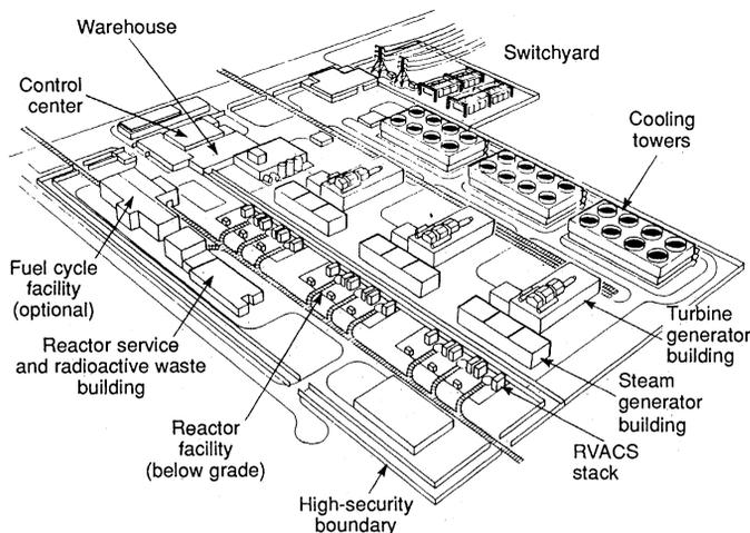
Fig. 4. PRISM 1395-MWe power plant.
