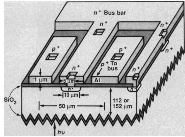
**Fig. 3.** Stanford University's innovative point-contact cell, which has exceeded all existing efficiency records for silicon cells. The device uses a textured front surface, oxide layers at the front and back surfaces, a highly reflective back surface, and an array of small, point-diffused emitter regions on the back of the cell. [Adapted from (80) with permission of the Institute of Electrical and Electronic Engineers, Inc., New York]
