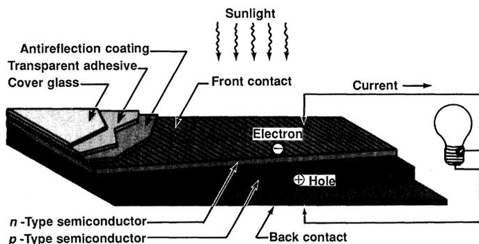
**Fig. 1.** In a typical PV cell, sunlight generates electron-hole pairs that are separated at the junction. This creates an internal voltage that drives current through an external circuit.
