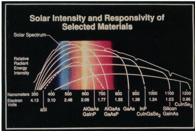
**Fig. 2.** The characteristic band gap of a semiconductor material is the energy level at which light of a particular wavelength, or shorter, interacts with the electrons in atoms of the material to produce electron-hole pairs, the onset of PV activity.
