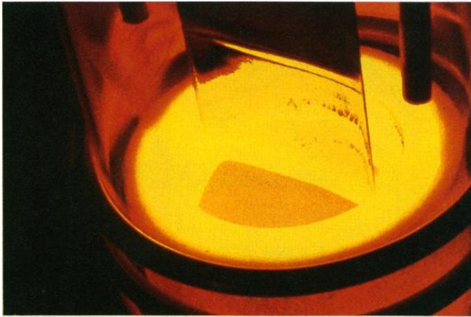
**Fig. 5.** One technique for making polycrystalline silicon PV cells is edge-supported pulling. With this process silicon sheets are crystallized from a liquid silicon meniscus, which is formed and stabilized between two parallel vertical graphite filaments immersed in the liquid.
