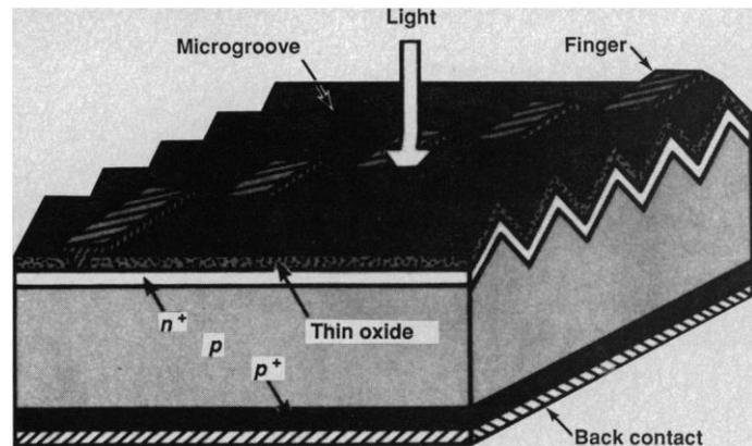
**Fig. 4.** Design of a new silicon cell devised at the University of New South Wales, Australia, that is expected to substantially improve silicon concentrator modules. The cell uses a microgrooved texture for the front surface, a thin layer of oxide to reduce recombination, and front and back contacts that allow the cell to be easily mounted in concentrator modules. [Adapted from (80) with permission of the Institute of Electrical and Electronic Engineers, Inc., New York]
