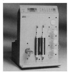
ylmethyloxycarbonyl polyamide active ester chemistry. Continuous flow synthesis produces peptides more quickly and with less reagent than synthesis by batch process; also, continuous flow synthesis allows online monitoring, if desired. Synthesis takes five steps, and washing, acylation, and deprotection steps are controlled from a keyboard. Pharmacia LKB Biotechnology (Sweden). Circle 467.
