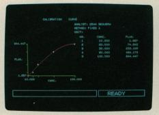
8:26 AM Quantitation Analysis Using a Higher Order Calibration Curve
