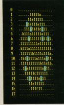
Optistation's automated wafer mapping capability ends the tedious physical counting of rows and searching for ink dots.
